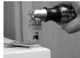
Angled ratchet screwdriver or socket wrench
